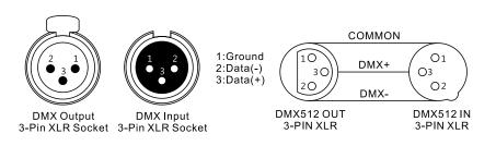
For installations where the DMX cable has to run a long distance or is in an electrically noisy environment, such as in a discotheque, it is recommended to use a DMX terminator. This helps in preventing corruption of the digital control signal by electrical noise. The DMX terminator is simply an XLR plug with a 120  $\Omega$  resistor connected between pins 2 and 3,which is then plugged into the output XLR socket of the last fixture in the chain. Please see illustrations below.
